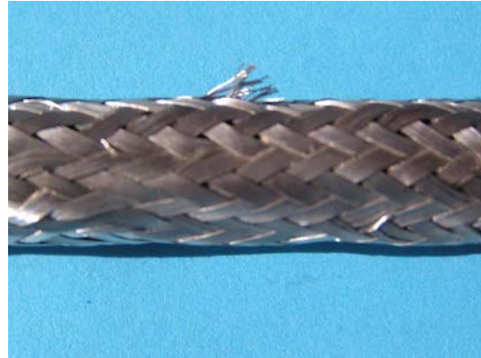
NOT ACCEPTABLE Damaged and Nicked Conductors
